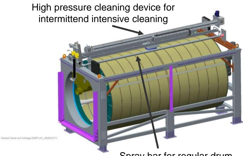
Spray bar for regular drum surface cleaning
